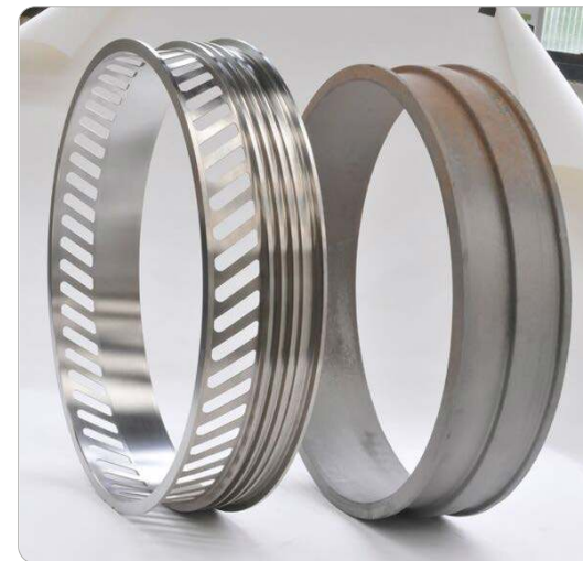
Reactor ring, calendered and welded then machined to very close tolerances for Airbus A320-330, Boeing 737, 747, 777 and 787 Image courtesy of Centro Inox
