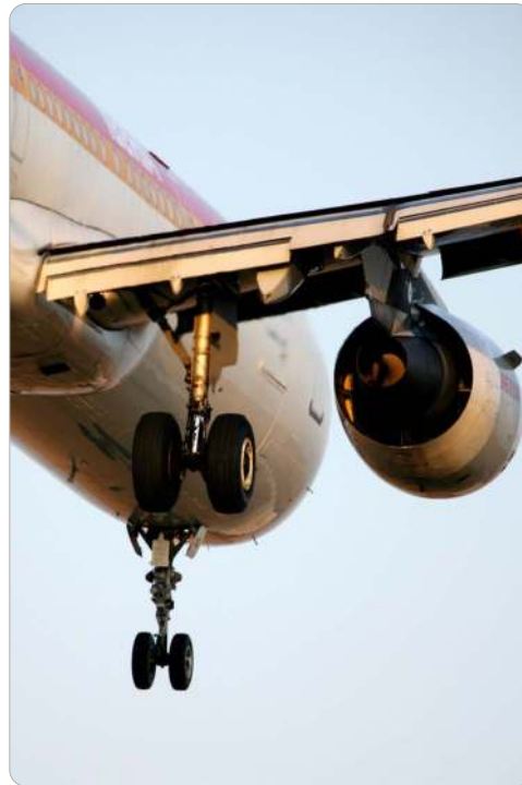
Landing gear components. Grades: EN: 1.4548 (AISI 630) re-melted and EN: 1.4545 (AMS 5659, ASTM 564). Picture courtesy of Iconos.
