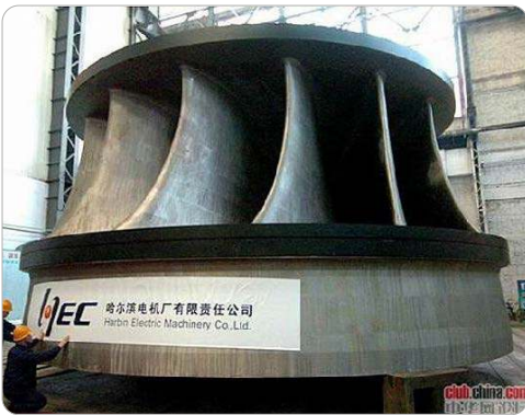
A turbine runner of the Three Gorges Power plant
