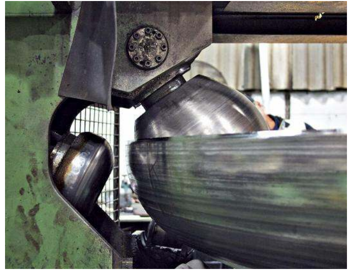
Spin forming of an austenitic stainless steel tank head takes advantage of the steel's high ductility. © IMO A
