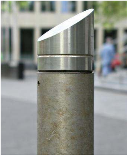
This Type 316 stainless steel bollard is exposed to road-salt splashing from passing cars. The bottom has a rough ground finish and the top a smoother polished finish which causes the performance difference. © IMO A
