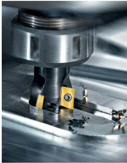
Side milling using carbide cutters. © Seco Tools
