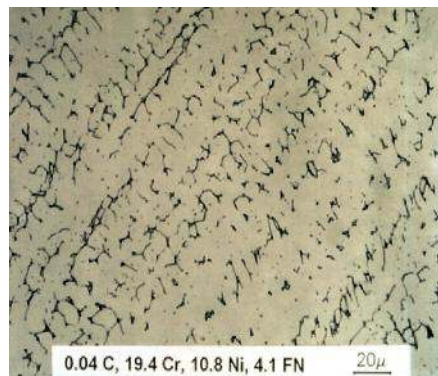
Austenitic stainless steel weld metal with different ferrite contents. © Lincoln Electric
