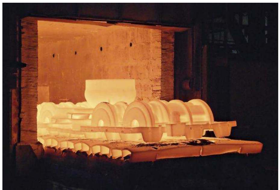
Batch heat treat process of stainless steel components. © Fondinox
