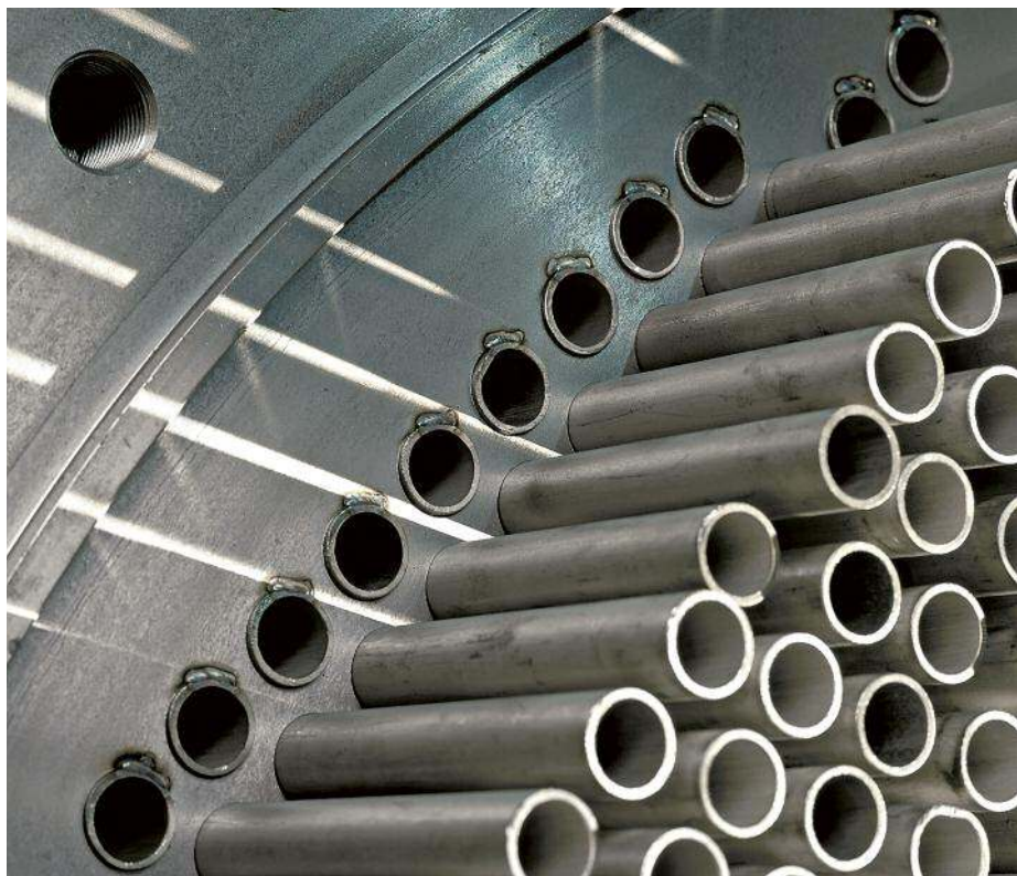
Heat exchanger tubesheet during fabrication. © Sandvik
