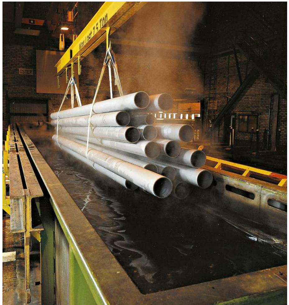
Degreasing of the surface is an essential cleaning step before any heat treatment. © Sandvik
