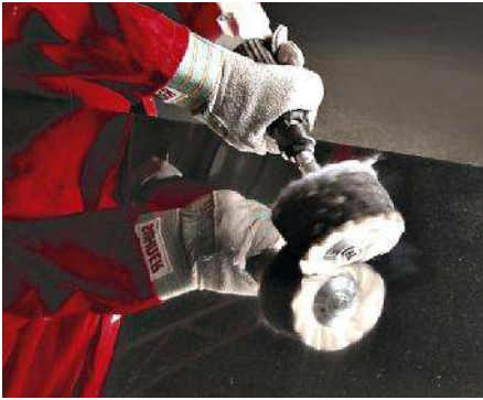
Buffing adds luster to a stainless steel surface. © Magic Disc
