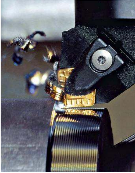
Turning stainless steel using carbide with a built-in chip breaker. © Seco Tools
