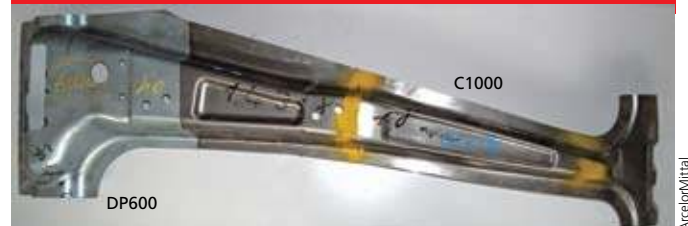
A B-pillar made of carbon steel DP600 and stainless steel C1000 was validated in a crash test during the NGV Project. The tailored laser-welded blank has a tensile strength of greater than 1000 MPa (145 ksi).
