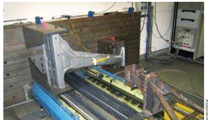
A B-pillar made of carbon steel DP600 and stainless steel C1000 was validated in a crash test during the NGV Project. The tailored laser-welded blank has a tensile strength of greater than 1000 MPa (145 ksi).
