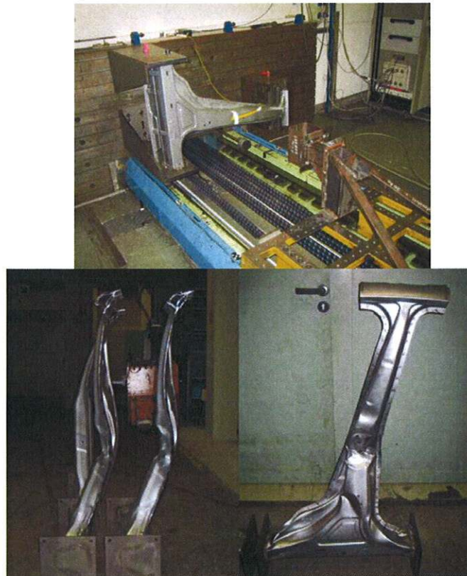
Fig 7 The crash test rig and the resulting component geometry after testing
